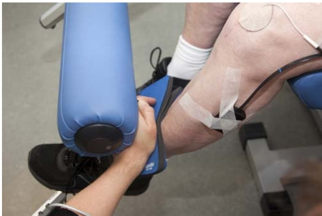
FIGURE 3 Picture of the experimental setup for the maximal isometric knee-extension strength measure using fixated handheld dynamometry.
